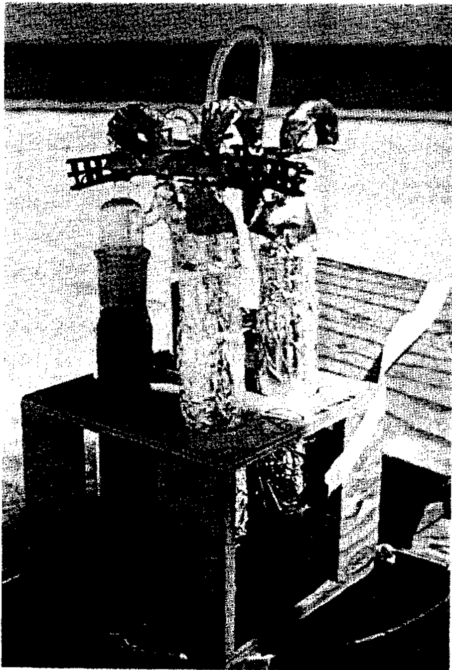
PLATE 7. BENZENE IMPINGER SETUP. BENZENE FLASKS ARE WRAPPED IN ALUMINUM FOIL TO PREVENT PHOTO-DECOMPOSITION OF TRAPPED SPECIES
