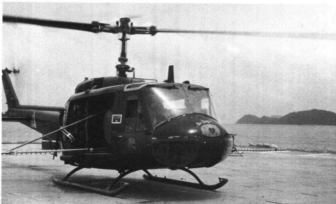
Fig. II B-3. UH-1D helicopter equipped to dispense herbicides. DOD (U.S. Army) photo taken in 1968.
